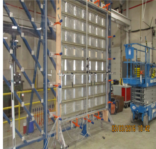
Specimen prepared for structural load testing
